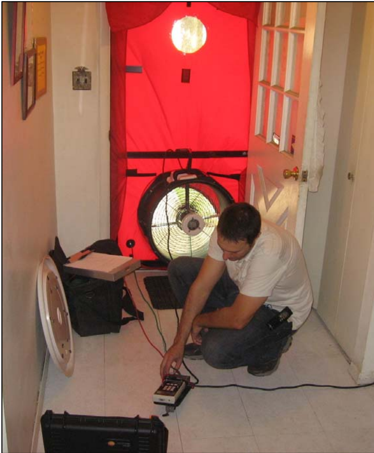
Rich Gajarsky from Avalon Energy Services performs both blower-door tests and thermographic inspections (infrared scanning) in GUIDE's client residences and main office.
